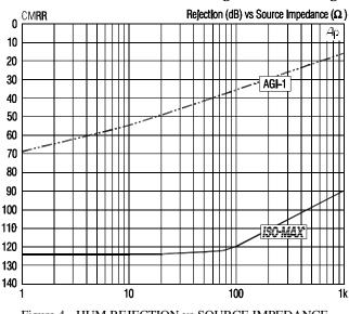
Figure 4 - HUM REJECTION vs SOURCE IMPEDANCE
