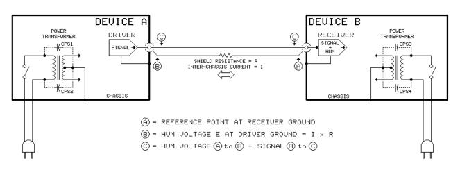
Figure 1 - THE HUM GENERATING MECHANISM The basic problem is that the shield is a common path for both inter-chassis "ground" and signal currents.
