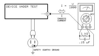
Figure 3 - MEASURING THE CHASSIS CURRENT
